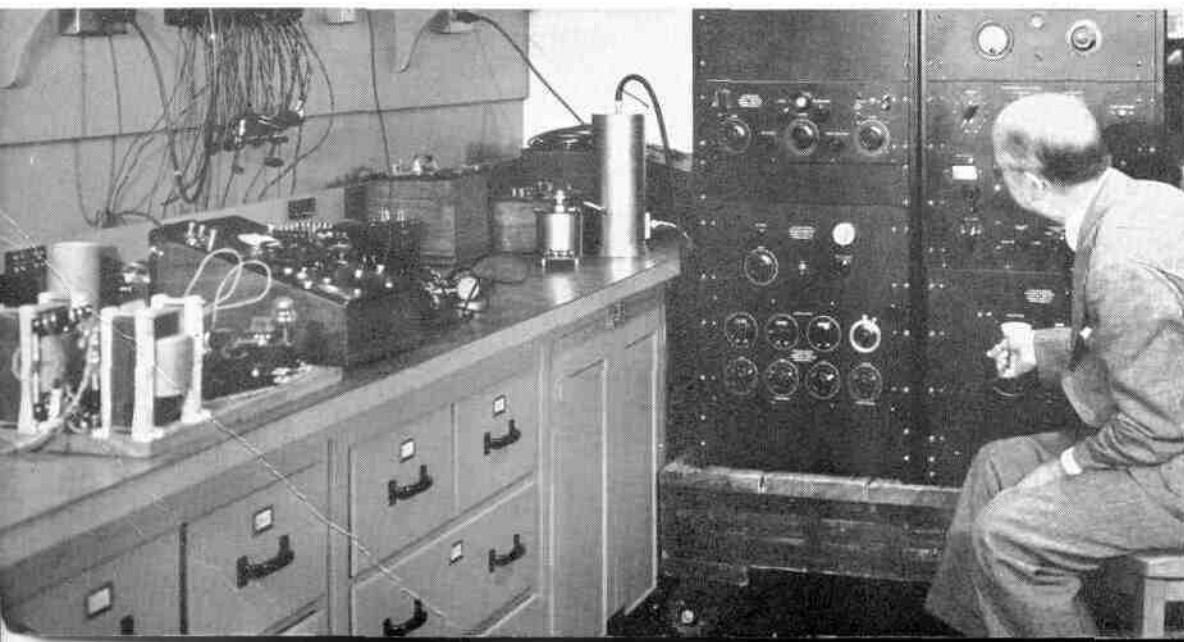
Below—Engineering tests on a high-voltage, 60-cycle Schering Bridge.
